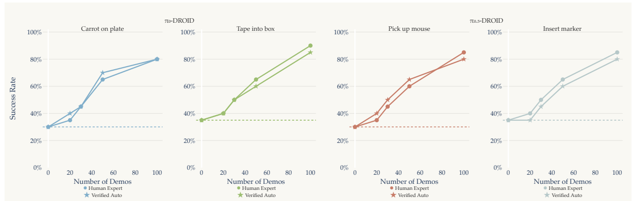
Figure 7 | Comparing data efficiency of autonomous verification v/s human expert. We fine-tune the base policy on datasets of 20, 30, 50, and 100 trajectories collected via either human expert teleoperation or verifier-curated autonomous rollouts, and evaluate each resulting policy over 20 real-world trials. Across all four tasks, verifier-curated data achieves comparable or superior data efficiency to human demonstrations. In multiple cases, autonomous data matches or outperforms human data at the same budget (e.g., 20–50 demos), and remains competitive even at larger scales. For example, on Pick up mouse , 50 autonomous demos outperform human demonstrations (0.65 vs. 0.60), while for Carrot on plate , performance is identical. These results indicate that verifier-curated autonomous collection can match the data efficiency of expert demonstrations, enabling scalable policy improvement without supervision.
